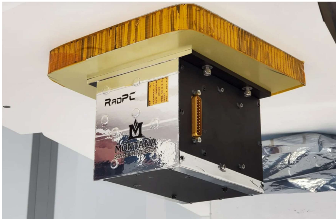
The RadPC prototype was photographed at Montana State University prior to being installed aboard the Blue Ghost lander. Credit: Firefly Aerospace
