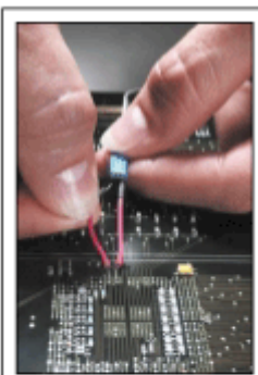
Figure 3 FPGA signals in a BGA package that were not brought out to a logic analyzer test point can still be observed using a damped-wire accessory and a flying
