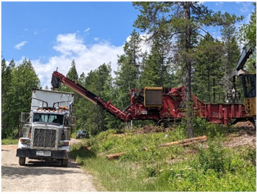
F.H. Stoltzes' B66 Rotochopper and chip van. (Photo courtesy of Matthew Bishop)
