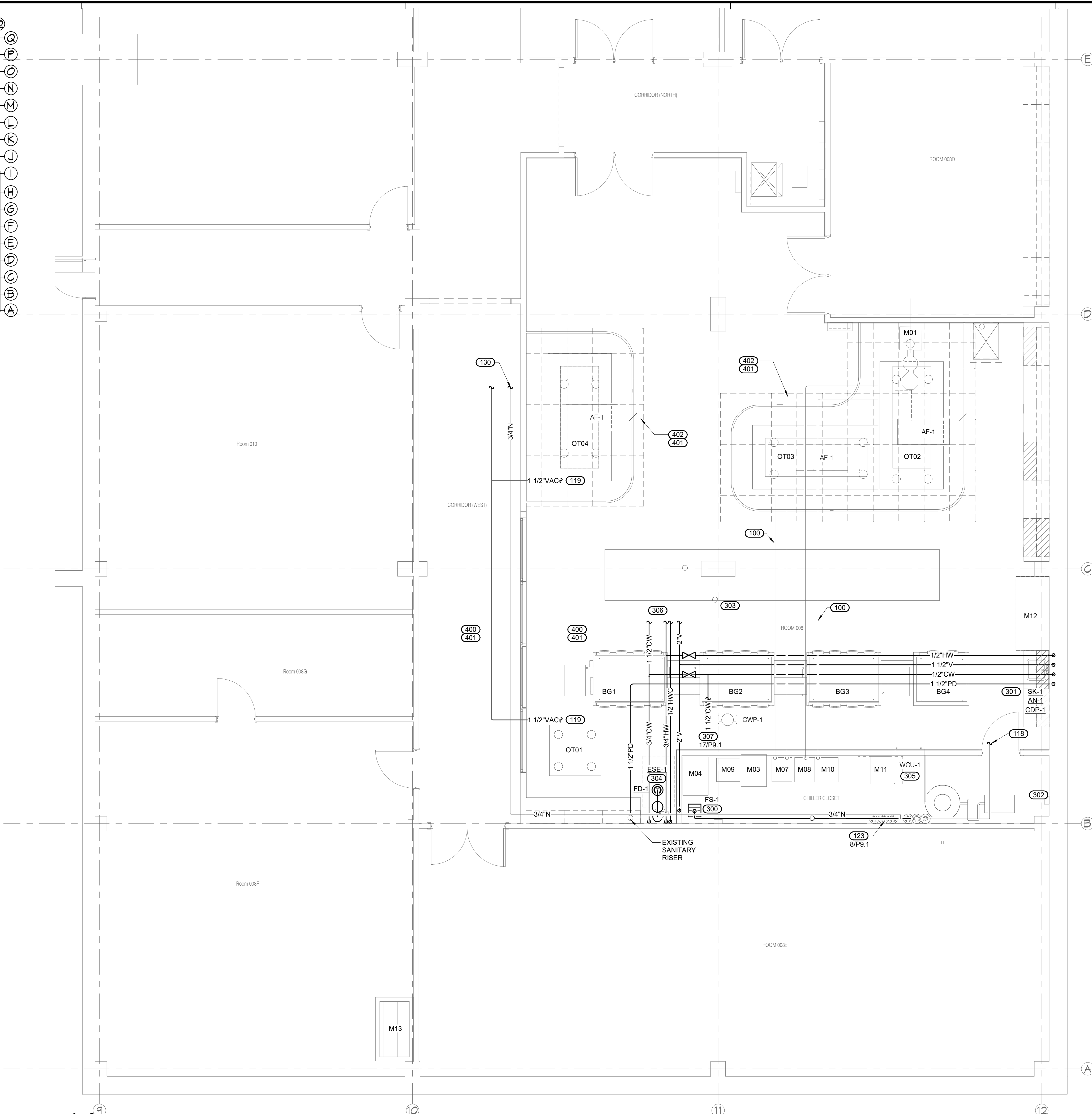
16 BASEMENT ROOM 008 PLUMBING PLAN P2.B 1/4" = 1'-0"
