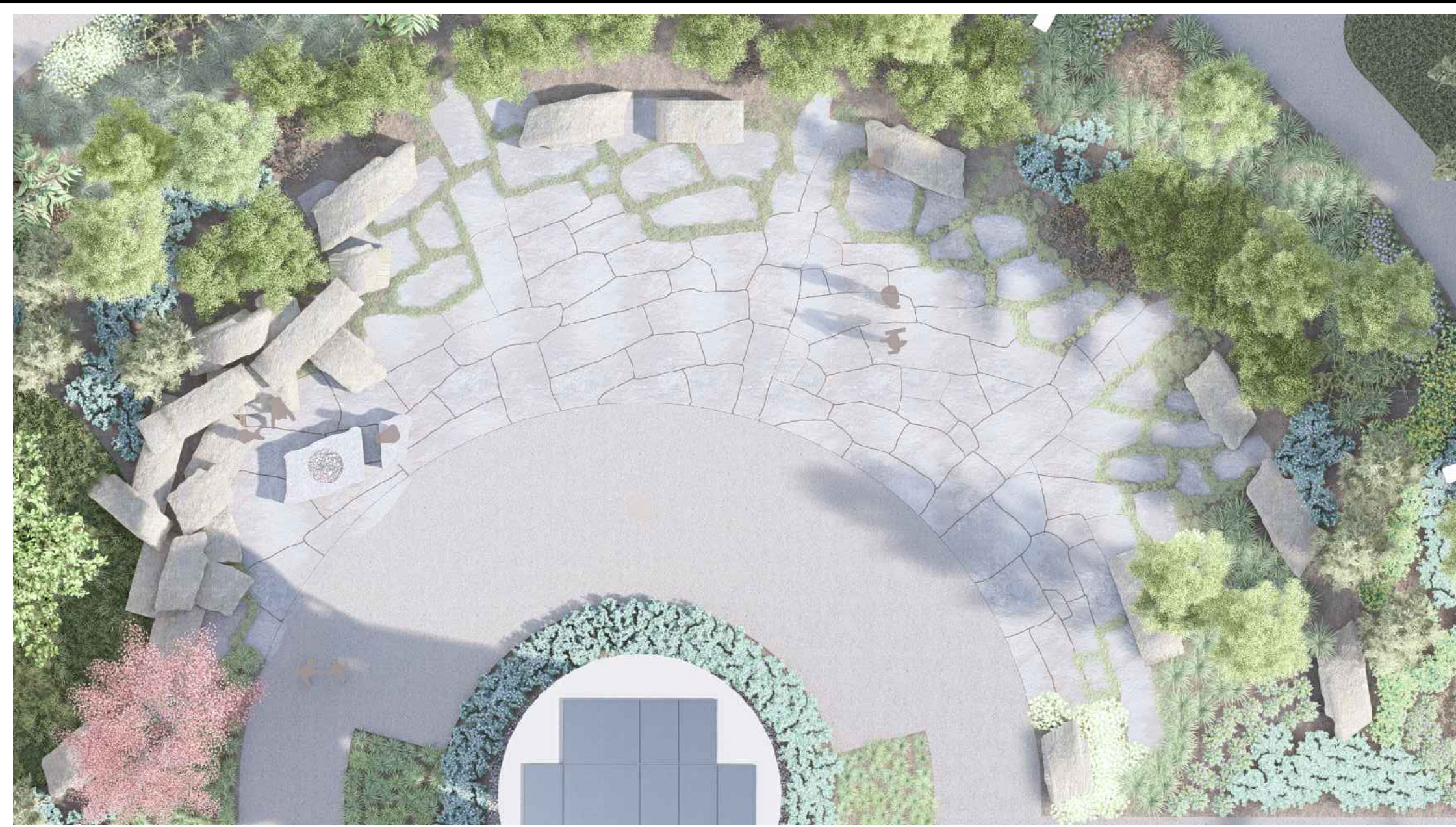
1 L7.0 Jumbo Format Windsor Gray Flagstone - Cut and Fit Layout Design Intent NTS
