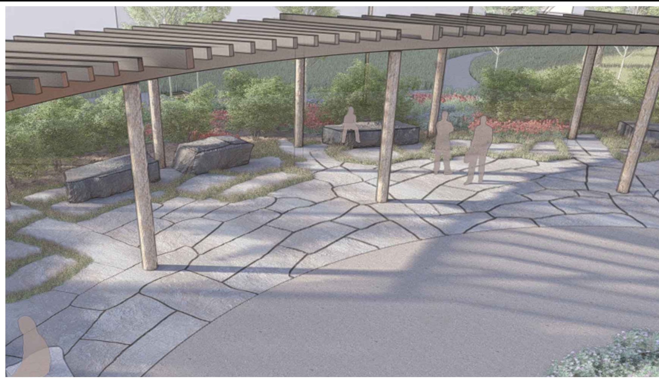
2 L7.0 Jumbo Format Windsor Gray Flagstone - Cut and Fit Layout Design Intent NTS
