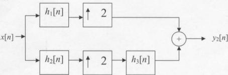
(b) If the three unit sample responses  $h_1[n]$ ,  $h_2[n]$ , and  $h_3[n]$  are all restricted to be zero outside the range  $0 \le 2$ , determine and explain your choices for  $h_1[n]$ ,  $h_2[n]$ , and  $h_3[n]$  so that  $y_2[n]$  is identical to  $y_1[n]$
