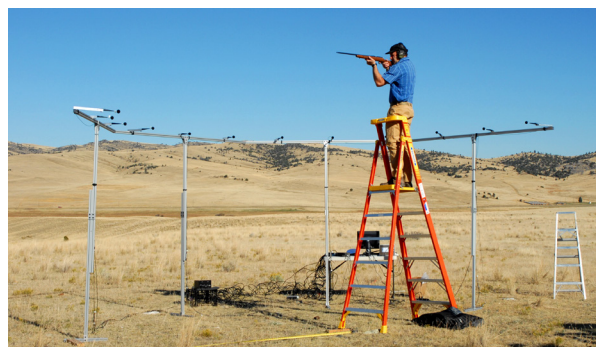
Figure 6: 3 m elevated structure to create a quasi-anechoic platform covering 180^\circ azimuth range.
